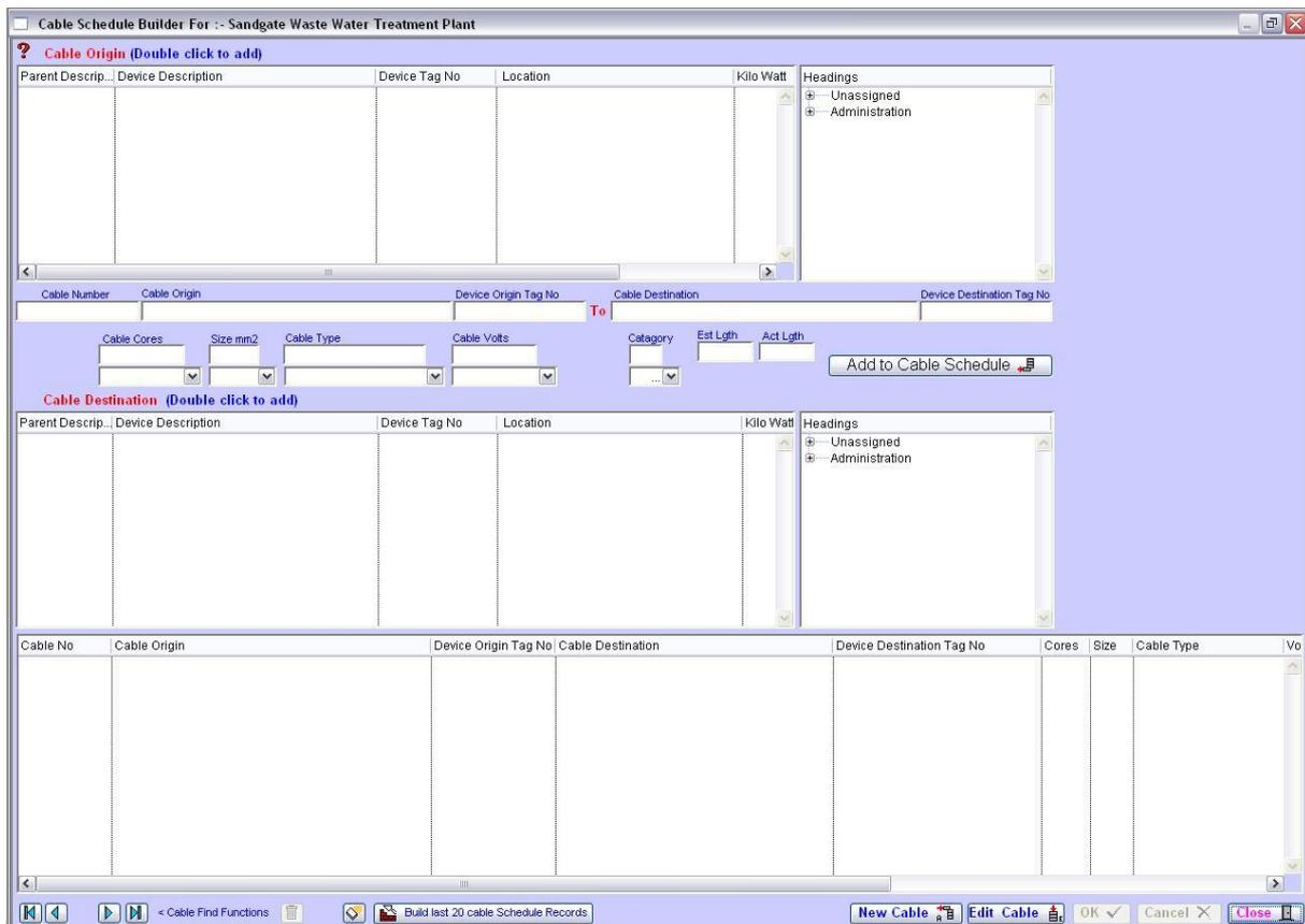
Generally to set a new cable schedule use the 'Cable Origin' at the top of the screen. Click 'New Cable'. Locate the 'Cable Origin' and then click on the 'New' button under the 'Cable Origin' screen. Select the 'Cable Destination' and then click on the 'Edit' button located on the top of the 'Cable Destination' screen.
